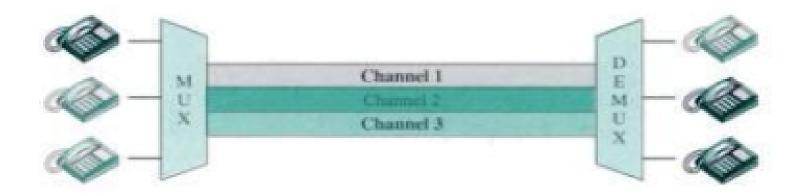
Transmission path is divided into three parts, each representing a channel to carry one transmission.
