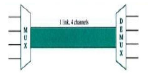
Link refers to the physical path, and channel refers to the portion of link that carries transmission between a given pair of lines. One link can have many channels.
